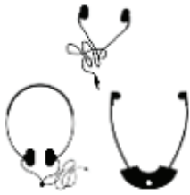
Figure 5: Top: A monaural ear-bud (not recommended but sometimes provided); Bottom: a standard stethoscope-type headset; Bottom: a specialized headphone with electronics built-in for infrared reception.
