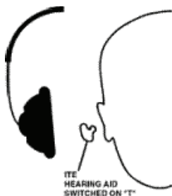
Figure 7: Coupling a hearing aid to an ALS by placing the headphone over the hearing aid while it is switched to the "T" setting.
